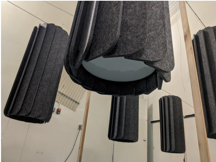
Figure 2 – Detail of specimen material, recessed acrylic lens, felt fins
